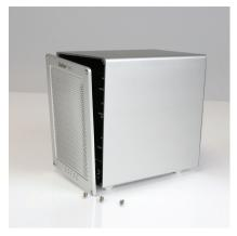
5. Using the included Allen key, drive each of the four screws back into the enclouse through the front place plate.
